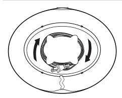
The base of the slow cooker is recessed to provide cord storage. After the unit is cool, remove the lid and crock. Turn the base upside down and wind cord as shown.
